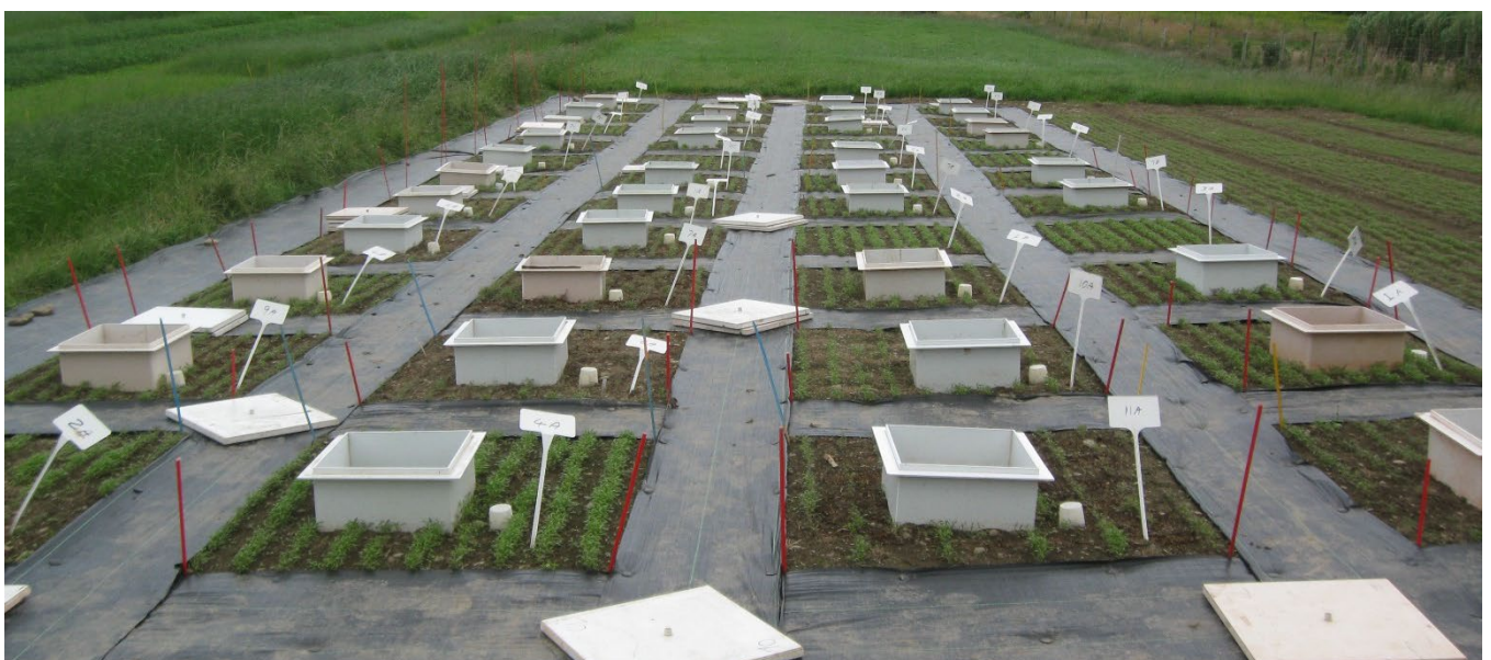
Field experiment at Bangor University showing gas collection boxes for nitrous oxide analyses
