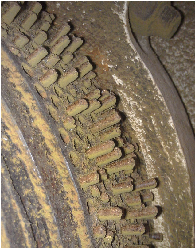
Alder pellets extruded in the Simon-Barron pellet mill
